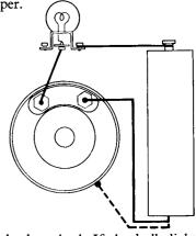
edges of the armature with the bare lead. If the bulb lights, this indicates a short circuit.
