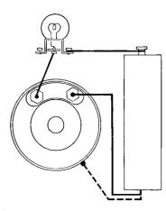
winding. If a test meter is not available, a battery and bulb may be connected as shown in the diagram, and if the bulb does not light a break in the armature winding is indicated. A second test is to disconnect the lead from one of the armature terminals and touch the outer edges of the armature with the bare lead. If the bulb lights, this indicates a short circuit.
